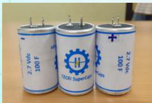
Symmetric cylindrical supercapacitor device fabricated using activated carbon developed at CSIR-CECRI.
